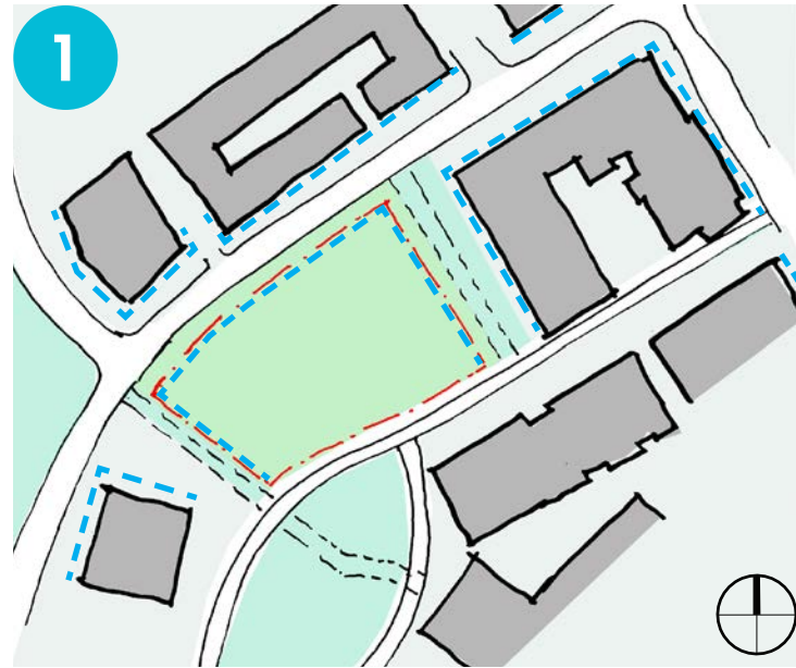
1 Load site perimeter with buildings to create street wall / urban village feel.
