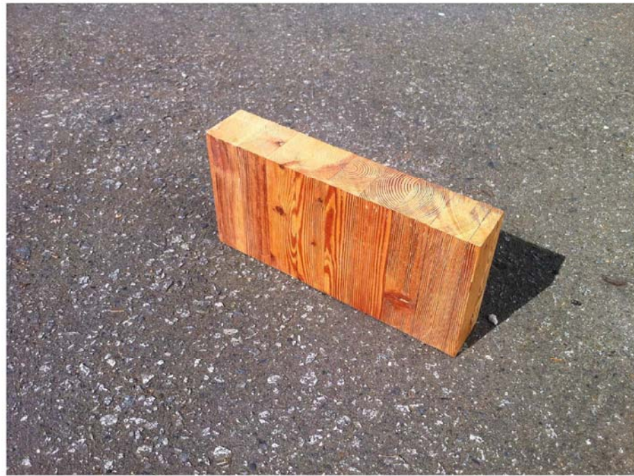
WOOD DECK (ROOF STRUCTURE AND INTERIOR CEILING)
