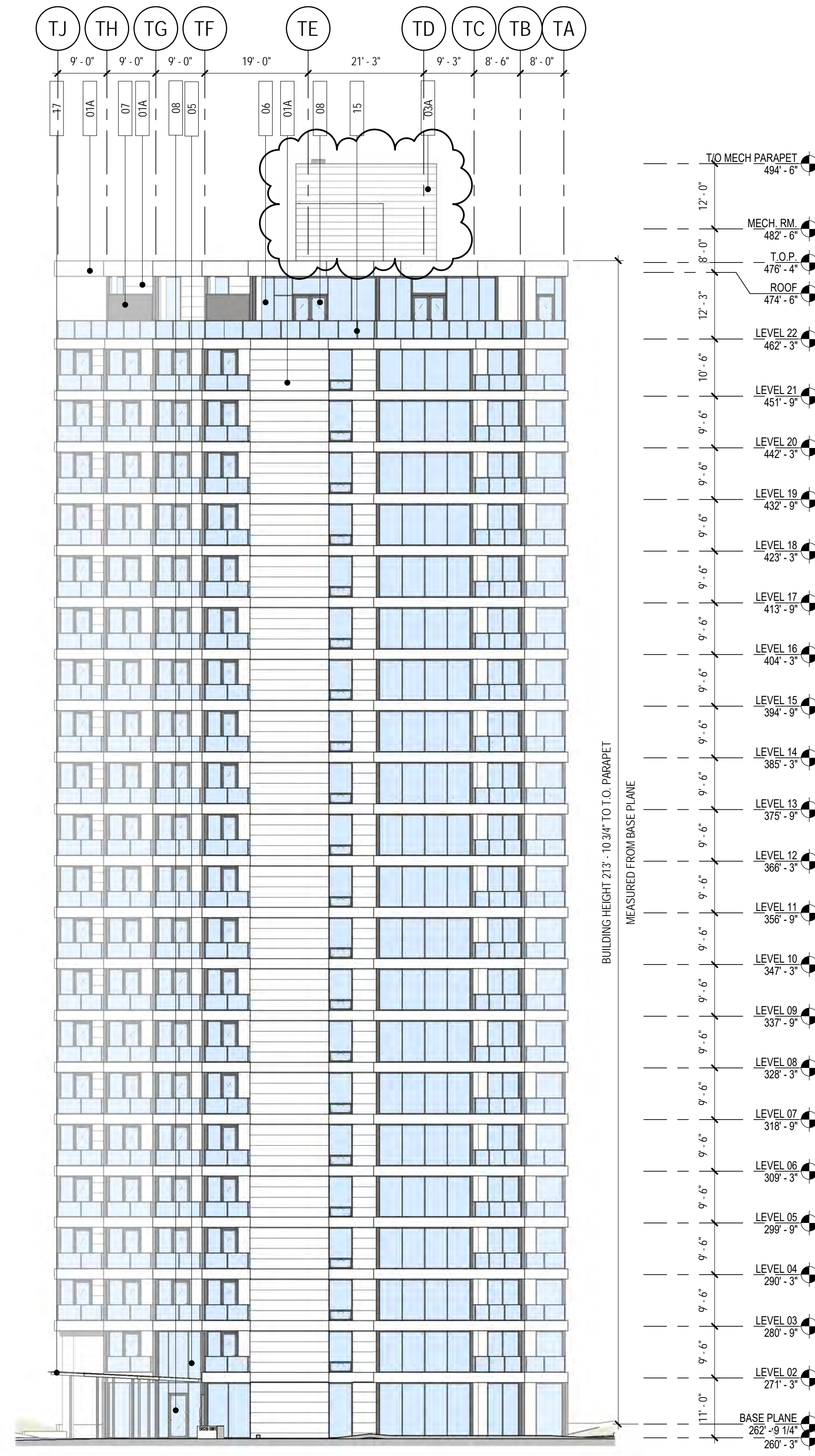
① TOWER SOUTH ELEVATION 1/16" = 1'-0"
