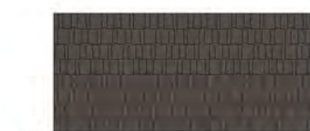
① ROOF : HEAVY PROFILE ASPHALT SHINGLES 'WEATHERWOOD'
