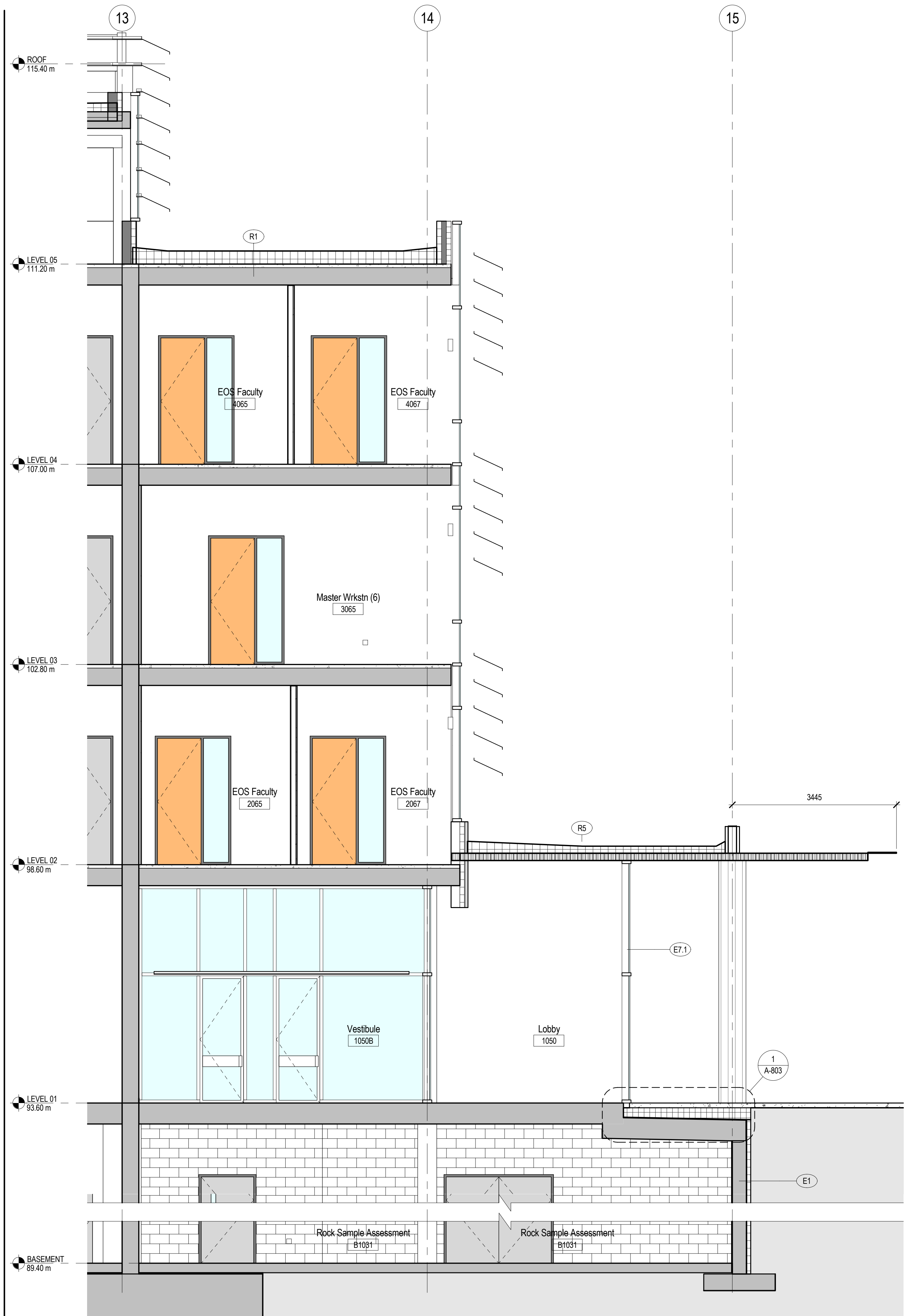
2 SOUTH - WALL SECTION - AT VESTIBULE 1:50
