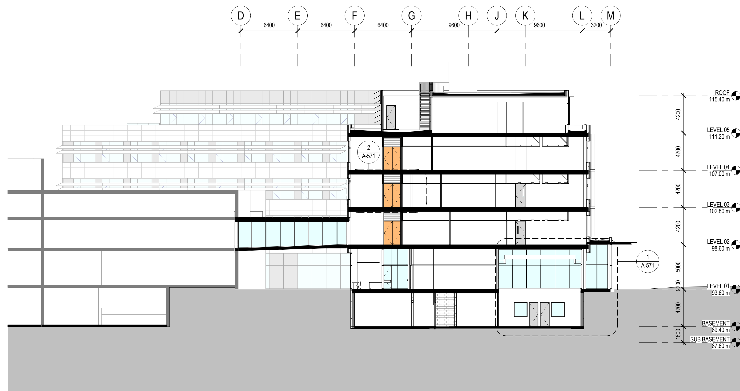
1 SECTION - SOUTH - BRIDGE CONNECTION 1:200
