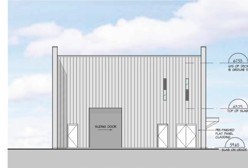
2 EAST ELEVATION C-05 1:100
