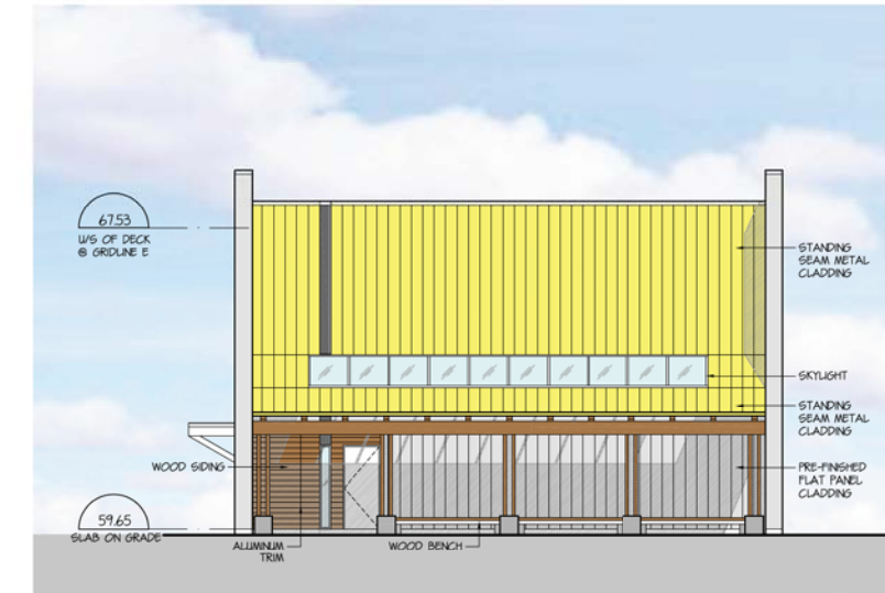
1 WEST ELEVATION C-05 1:100
