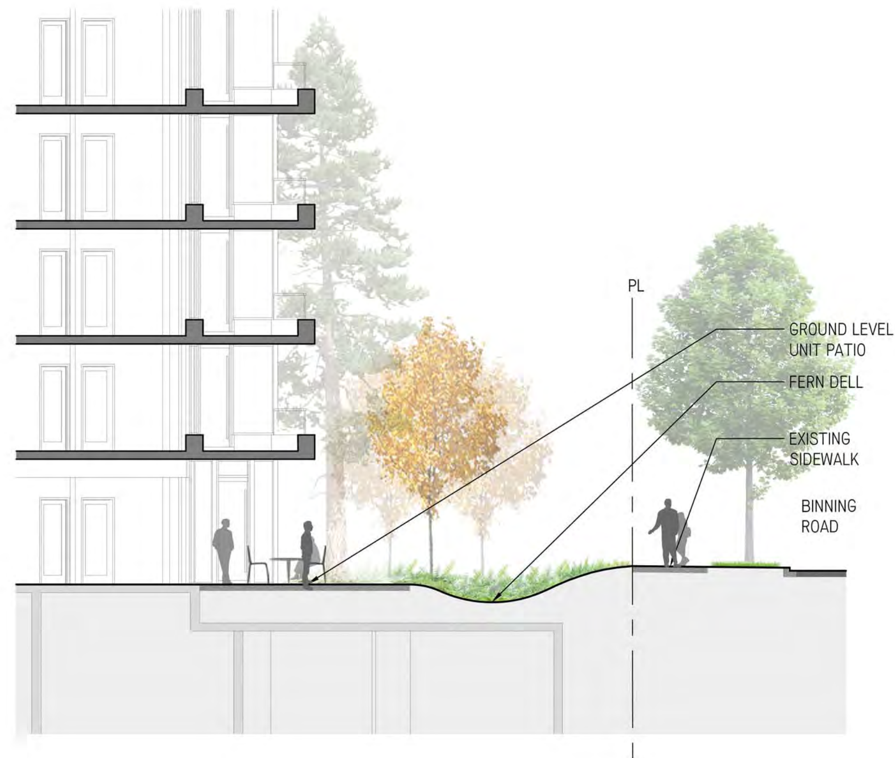
1 SECTION LOOKING NORTH THROUGH FERN DELL L2.10 1/8" = 1'0"
