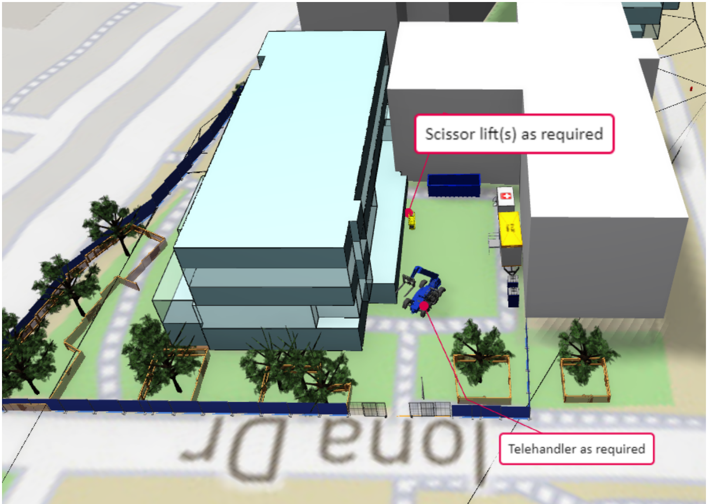
Figure 5 – Envelope & Finishes Structure Site Logistics Plan
