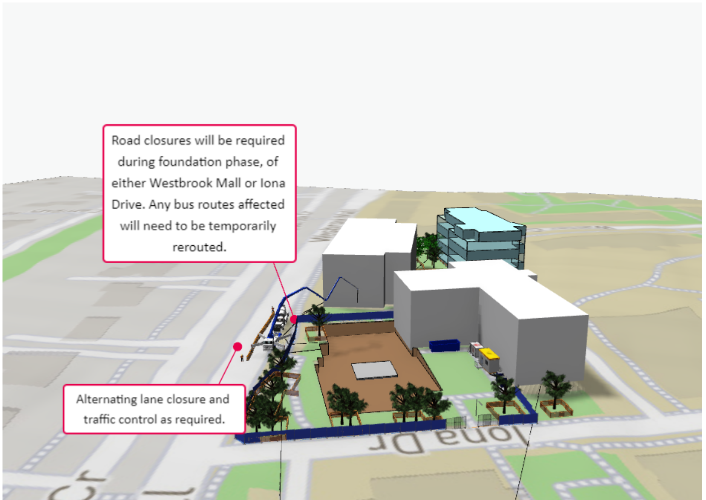
Figure 3 – Foundations Site Logistics Plan
