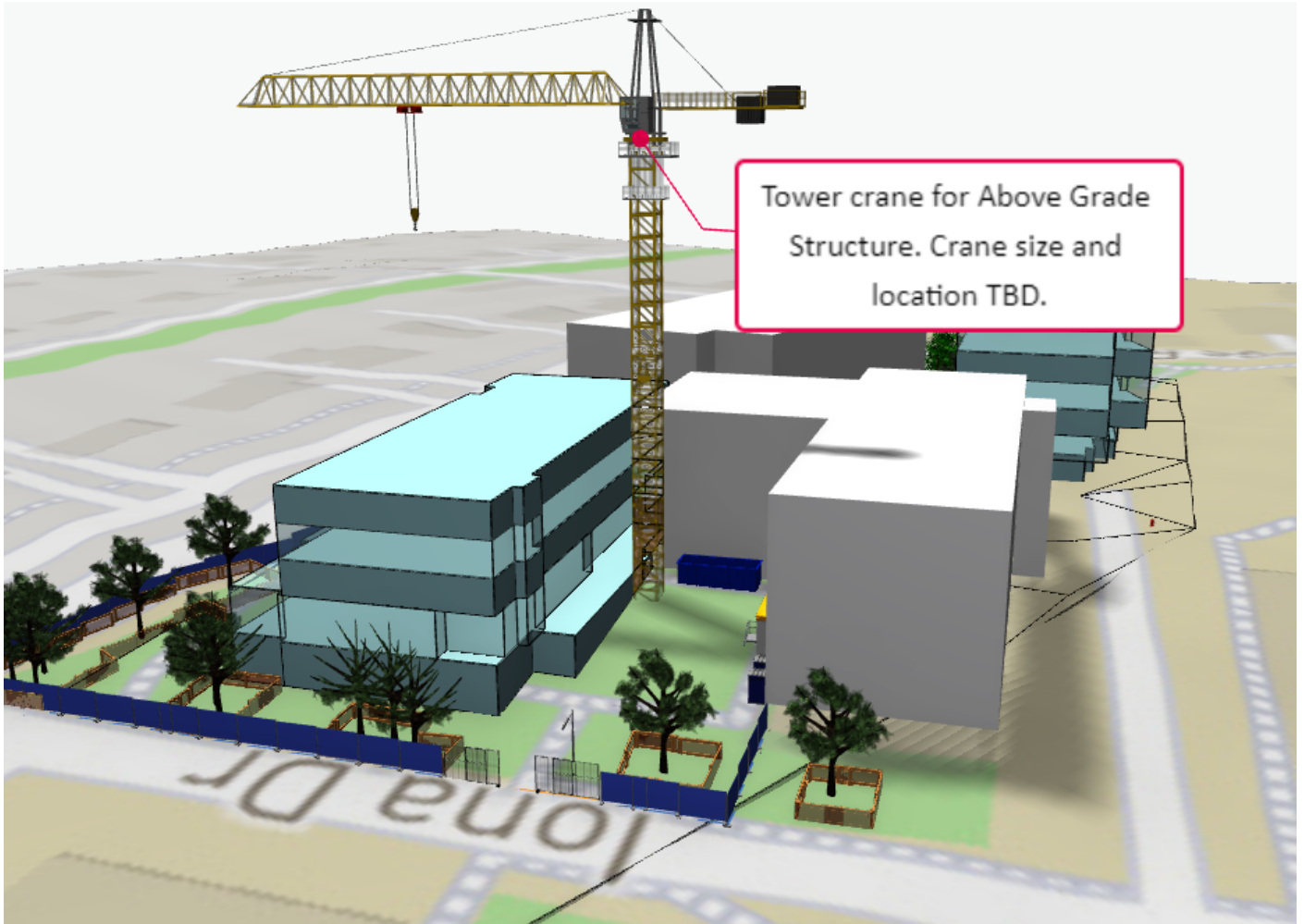
Figure 4 – Above Grade Structure Site Logistics Plan
