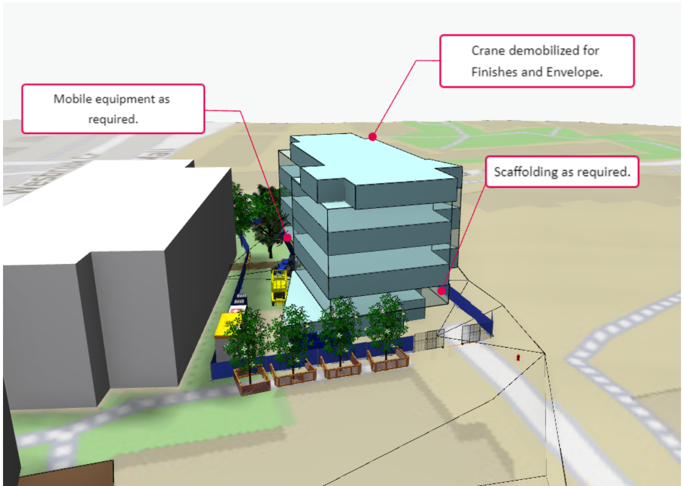
Figure 4 – Envelope & Finishes Structure Site Logistics Plan
