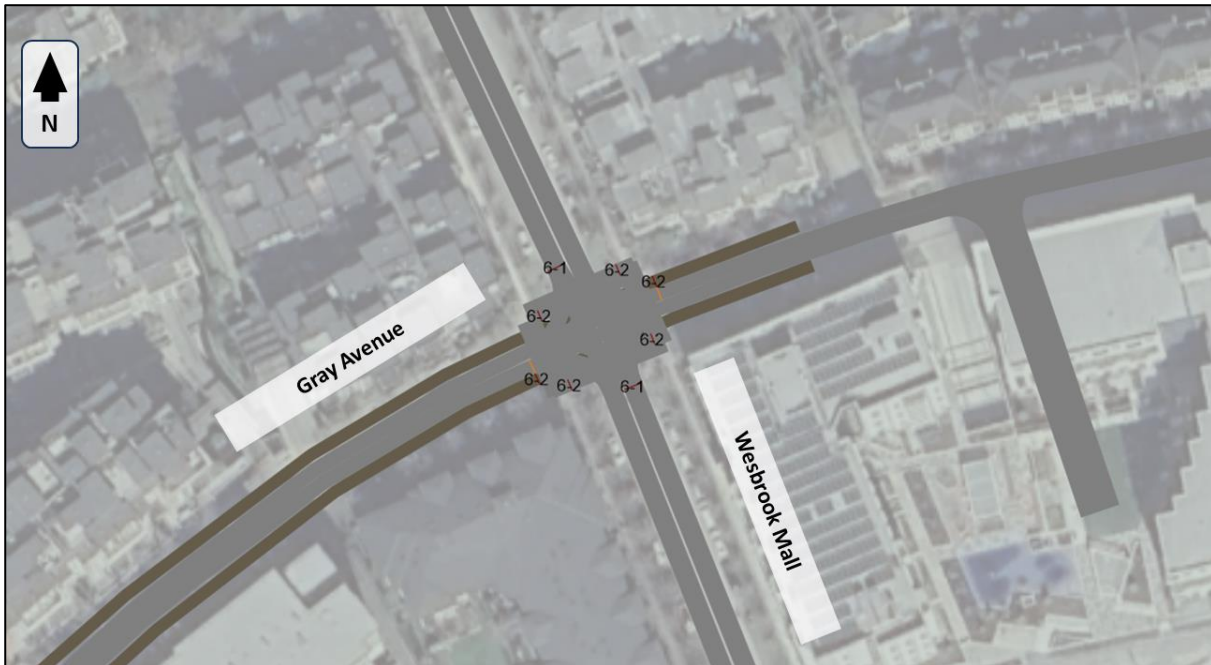
Figure 6.8: New pedestrian / bicycle signal at Gray Avenue and Wesbrook Mall
