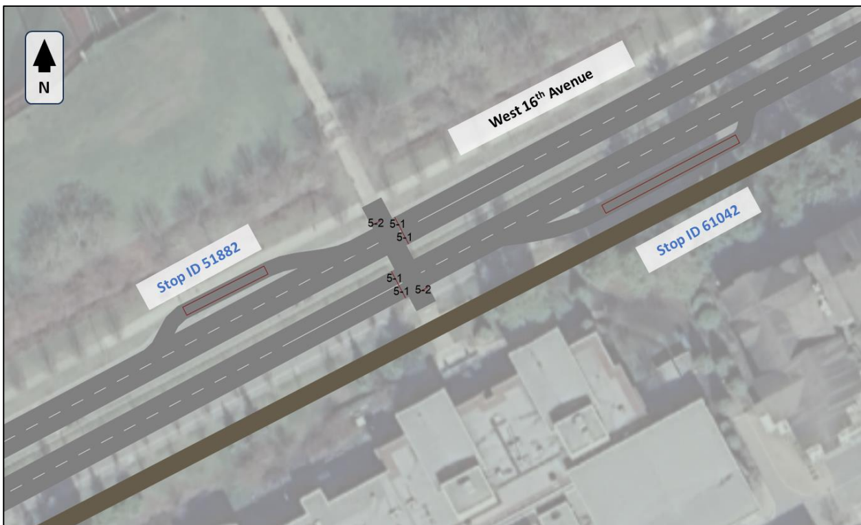
Figure 6.6: New mid-block pedestrian signal on West 16th Avenue
