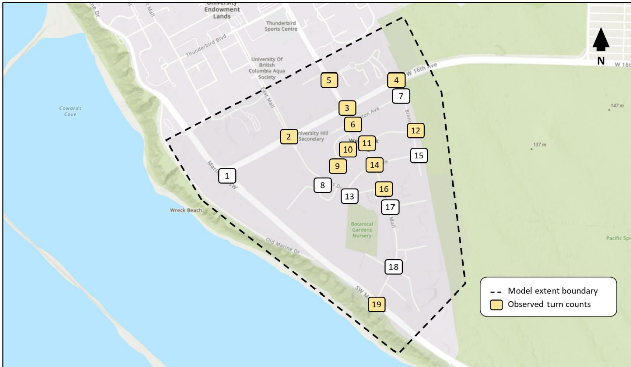
Figure 5.3: Summary of observed turn movement counts for intersections in the study area
