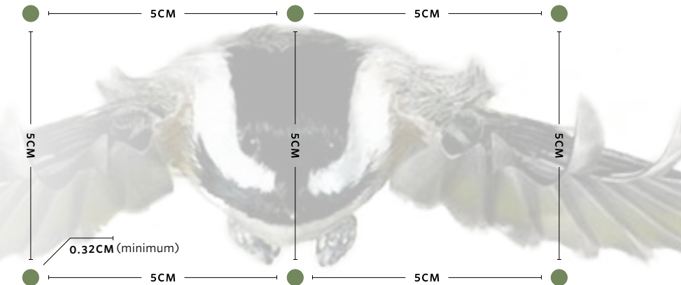
[FIG 1] Diagram of bird friendly glazing pattern with visual markers at maximum 5cm x 5cm spacing IMAGE SOURCE: FLAP CANADA
